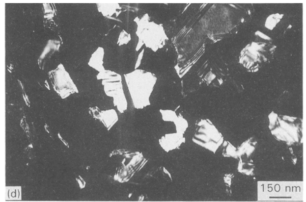
Figure 2 (a) Bright-field cross-sectional TEM micrograph of a MOVPE GaAs/Si (111) interface of GaAs grown on (111) Si at 650°C for 120 s. The electron beam is close to the (1\bar{1}1) . (b) Bright-field planar view TEM micrograph of a GaAs layer grown on Si (111) at 650°C for 120 s, and (c) corresponding SAD pattern. The electron beam is close to the (\bar{1}\bar{1}\bar{1}) . (d) Dark-field planar view TEM micrograph, obtained from a secondary twin spot, indicated by A in (c).
